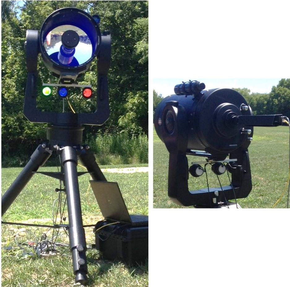
**Figure 31: 30.5 cm diameter color WFS transmitting green, blue, and red eyesafe LEDs (left). Rear view of the same color WFS with the optical train visible (right).**
